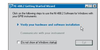
Caution Ensure the GPIB devices and the computer containing the GPIB-USB interface share the same ground potential. For help installing your hardware, refer to the *GPIB Hardware Guide* (available on the CD through **Getting Started Documentation**).
